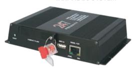
Key installed) can access the TVS21 to view and to retrieve recorded images. The TVS21 can upload to the Police notebook PC or the Police office PC via a network cable at the rate of more than 3000 images per minute.
