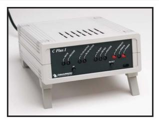
The *C Plus I* ANI computer interface unit is a compact, economical means to convert and forward ANI, Emergency, and Man-Down messages to a users computer. The *C Plus I* has a built in encoder providing automatic EM acknowledgements. The acknowledgement eliminates repeat Emergency transmissions.
