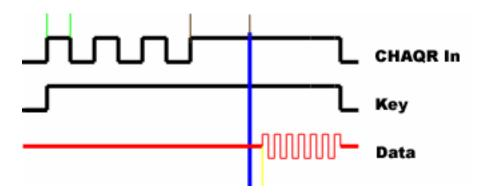
In this timing chart, the distance between green lines is 100mS, between brown lines is 250mS and from the Blue to the Yellow line is 50mS. The C Plus is programmed for *CHAQR* active High, *Attack Delay* of 50mS, *Trunk Debounce* of 250mS and *Trunk Key Time* and *Trunk Timeout* is set to 3 Seconds.
