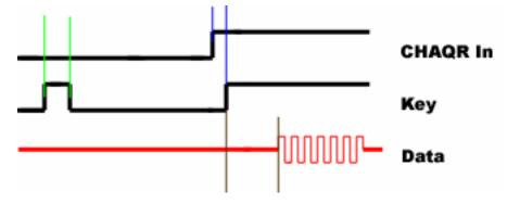
In this timing chart, the distance between green lines is 100mS, between blue lines is 50mS and between brown lines is 200mS. The C Plus is programmed for *CHAQR* active High, *Attack Delay* of 200mS, *Trunk Debounce* of 50mS, *Trunk Key Time* of 100mS and *Trunk Timeout* to 3 Seconds.
