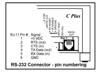
The +5 VDC is to power a Cimarron CDT. Jumper JP-2 must be installed to connect pin 1 to the fused (1A) +5 V source.
